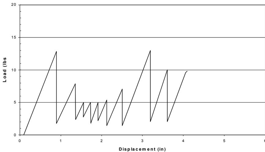
Fig. 4. Trousers test – loading rate 5mm/min
