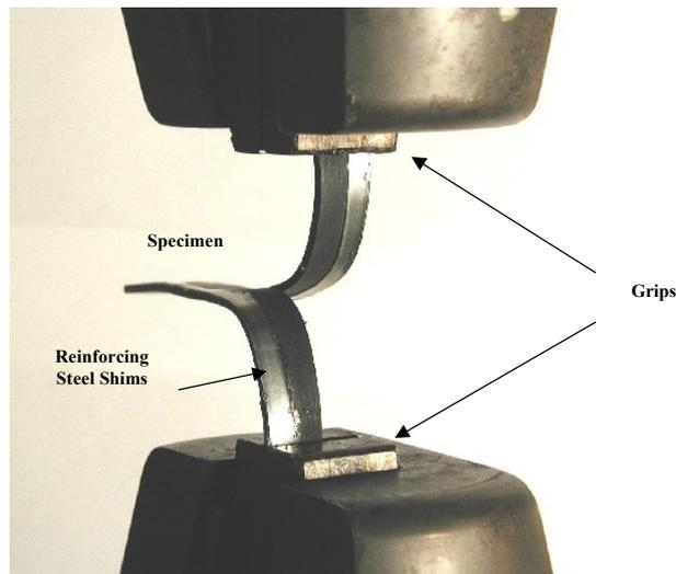
Fig. 3. Trousers Test Setup – Specimen with Steel Shims
