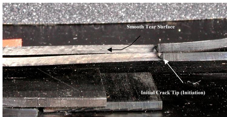
Fig. 9. Image of tear surface from constrained tension test
