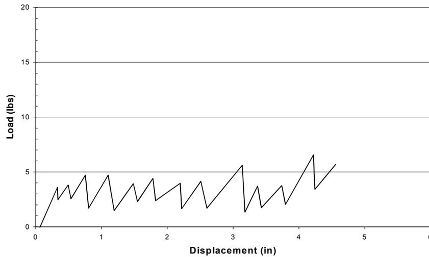
Fig. 7. Trousers test – loading rate 3.0 in/min
