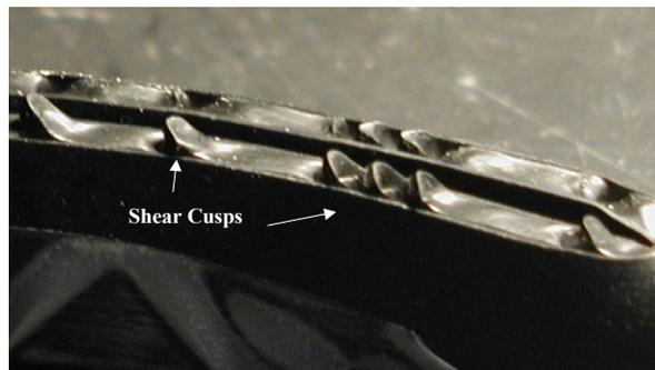
Fig. 5. Image of knotty tear surface
