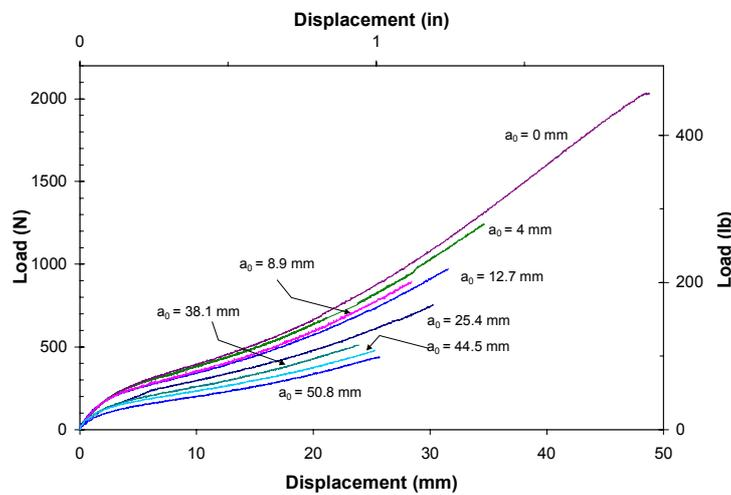
Fig. 8. Load vs. Displacement Curves for Constrained Tension Specimens for Different Crack Lengths
