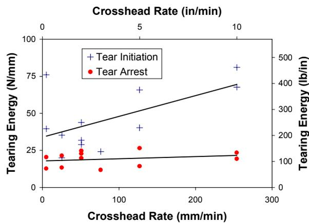
Fig. 10. Effect of loading rate on the initiation and arrest tearing energies
