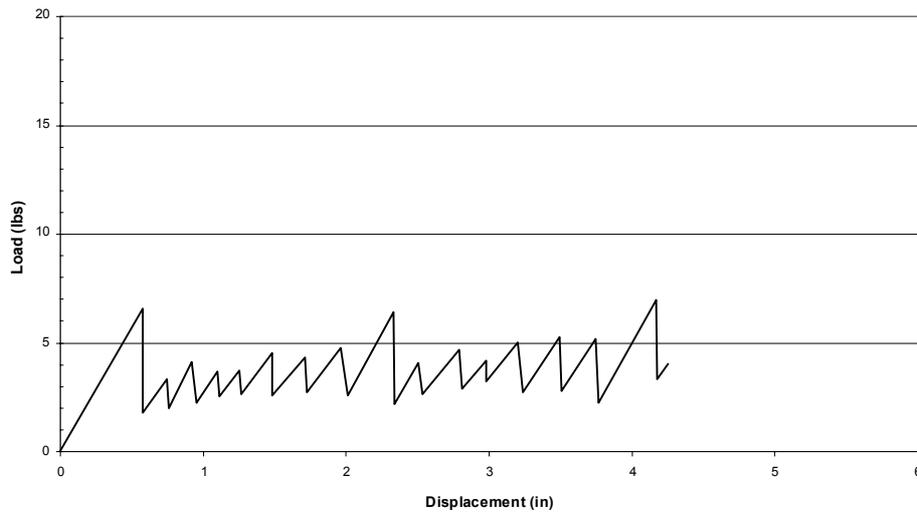
Fig. 6. Trousers test – loading rate 1 in/mm
