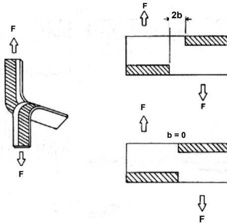
Fig. 1. Trousers Specimen with Shim
