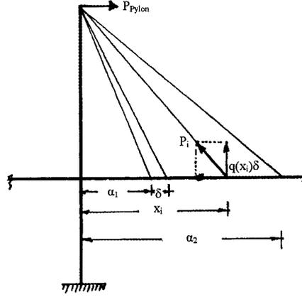
Fig. 3. The load  $q(x)$ , which expresses the effect of the cables on the bridge deck.
