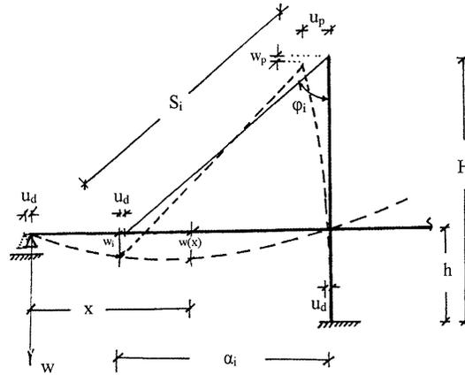
Fig. 4. Deformation of the girder. Cables at the left of the pylon.
