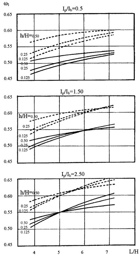
Fig. 9. Relationship between the first eigenfrequency  $\omega_1$  and the ratio  $L/H$  for various values of  $h/H$ .
