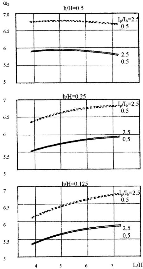
Fig. 8. Relationship between the first eigenfrequency  $\omega_3$  and the ratio  $L/H$  for various values of  $I_p/I_b$ .
