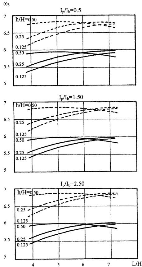
Fig. 11. Relationship between the first eigenfrequency  $\omega_3$  and the ratio  $L/H$  for various values of  $h/H$ .
