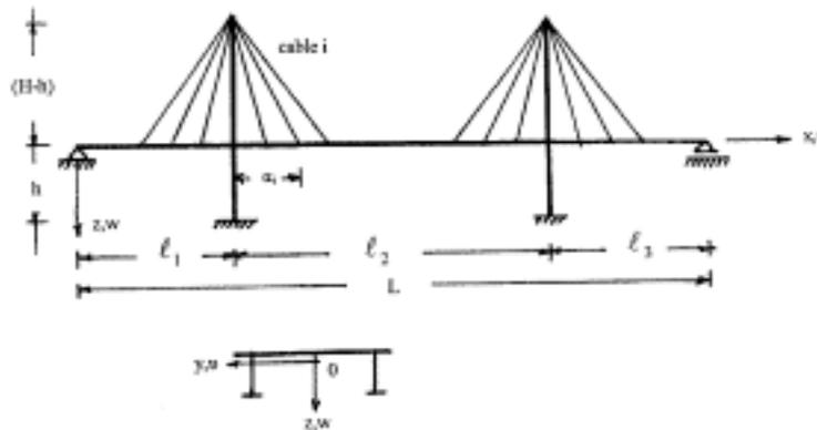
Fig. 1. Structural scheme of a cable stayed-bridge.
