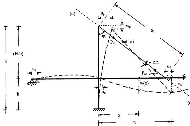
Fig. 2. Deformation of the girder. Cables at the right of the pylon.
