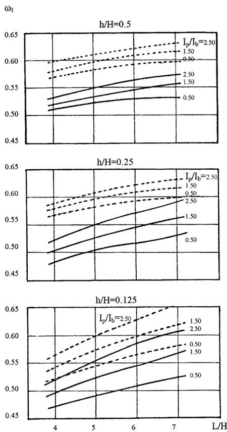
Fig. 6. Relationship between the first eigenfrequency  $\omega_1$  and the ratio  $L/H$  for various values of  $I_p/I_b$ .
