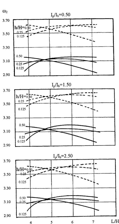
Fig. 10. Relationship between the first eigenfrequency  $\omega_2$  and the ratio  $L/H$  for various values of  $h/H$ .
