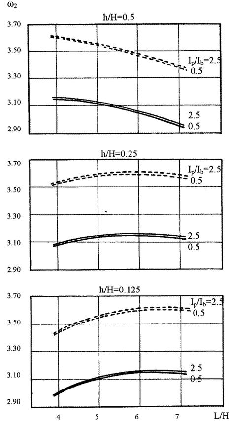
Fig. 7. Relationship between the first eigenfrequency  $\omega_2$  and the ratio  $L/H$  for various values of  $I_p/I_b$ .
