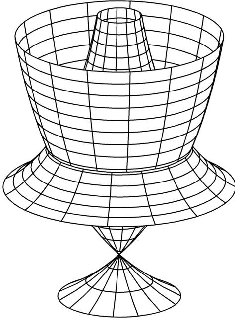
Fig. 3. Pseudo-sphere and parallel surface
