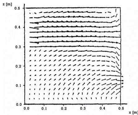
Fig. 2. Measured mean velocity vectors in a symmetry plane of the cubic box through the centers of both inlet and outlet windows
