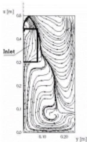
Fig. 6. Predicted streamlines in y-z plane at a distance of 8,75 cm from inlet opening
