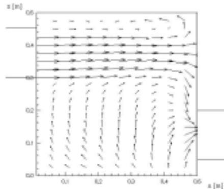
Fig. 3. Predicted mean velocity vectors in a symmetry plane of the cubic box through the centers of both inlet and outlet windows
