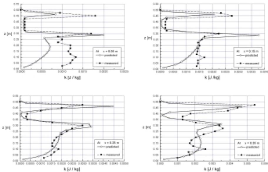
Fig. 8. Downstream change of turbulence kinetic energy in  $x$ - $z$  symmetry plane of the cubic box
