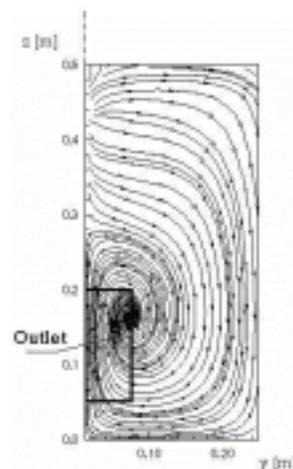
Fig. 7. Predicted streamlines in y-z plane at a distance of 11,25 cm from outlet opening
