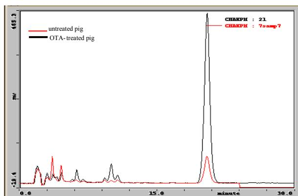
Fig. 2. HPLC profile of OTA and associated fluorescent compounds isolated from kidney of male pigs with and without added OTA
