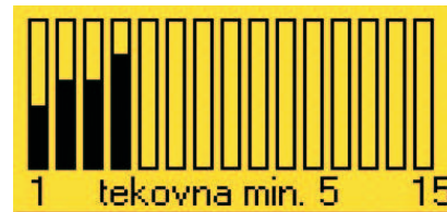
Fig. 10. "Chart" screen appears after we chose which parameter we want to view as a chart. Values of the parameter and the current minute are displayed.
