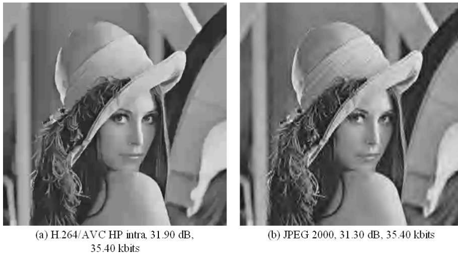
Fig. 7. Lena monochrome images comparing H.264/AVC HP intra coding (a) and JPEG 2000 coding (b) with 35.40 kbits per image.
