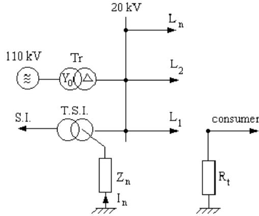
Fig. 1. Single-line diagram of the faulty network.
