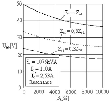
Fig. 3. Zero-sequence voltage as function of the fault resistance for a reactor-grounded network, operating at resonance.
