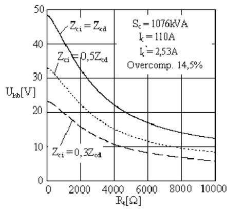
Fig. 4. Zero-sequence voltage as function of the fault resistance for a reactor-grounded network, operating overcompensated 14.5%.
