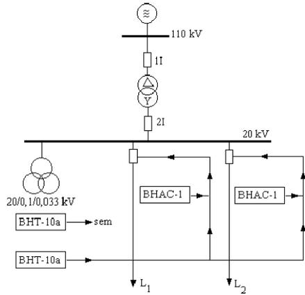
Fig. 7. Implementation of the BTH and BHAC protections in a medium-voltage network.
