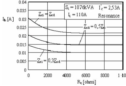
Fig. 8. Zero-sequence current as function of the fault resistance for a reactor-grounded network, operating at resonance.
