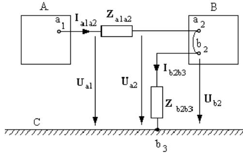
Fig. 2. Equivalent circuit of the faulty network.
