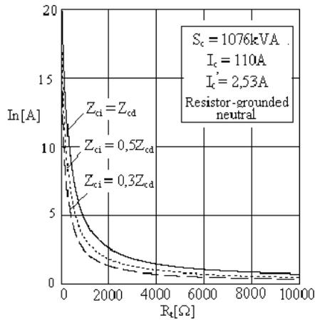
Fig. 6. Grounding current as function of the fault resistance for a resistor-grounded network.
