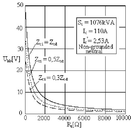
Fig. 5. Zero-sequence voltage as function of the fault resistance for a not-grounded network.
