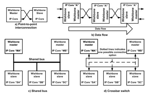
Fig. 5. Possible Wishbone interconnections
