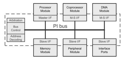
Fig. 8. TModules of a PI bus connected system
