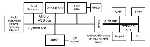
Fig. 1. AMBA based system architecture.
