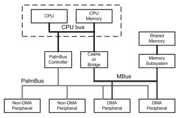
Fig. 6. CoreFrame architecture based system structure
