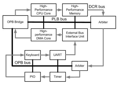
Fig. 3. CoreConnect bus based system
