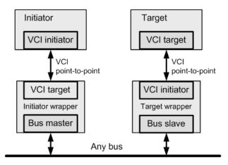
Fig. 11. Two VCI Connections Used to Realize a Bus Connection
