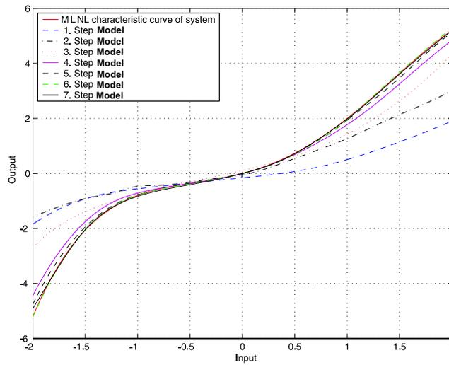
Fig. 5. Iterative convergence of identified MLNL sub-model
