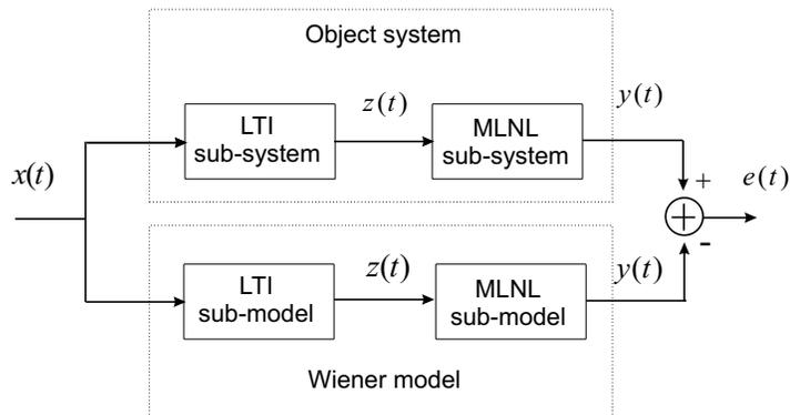
Fig. 1. System identification using Wiener model
