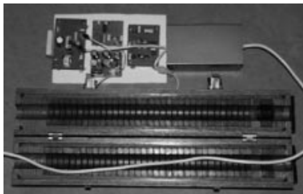
Fig. 4. Compartment with detector used for conducted EMI measurement.
