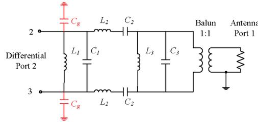
Fig. 2 Lumped-element representation of a balanced input third-order reconstruction filter with parasitic capacitances to ground  $C_g$  at the filter input
