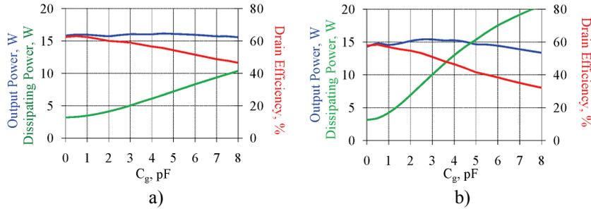
Fig. 5 ADS simulation results of the CMCD PA system operating at 450 MHz (panel a) and the CMCD PA system operating at 900 MHz (panel b): Drain efficiency (red curve), output power (blue curve) and power dissipated in the switch (green curve) as functions of the parasitic capacitance to ground  $C_g$
