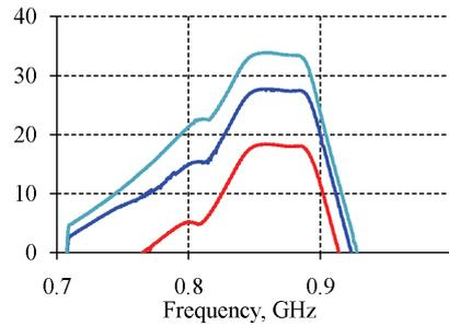
Fig. 8 Typical result for the measured output power of the class-S PA with a ST reconstruction filter, operating for test purposes in class-D over the specified bandwidth around 900 MHz centre frequency: for different biasing voltages of 2 V (red curve), 7 V (blue curve) and 15 V (light blue curve)
