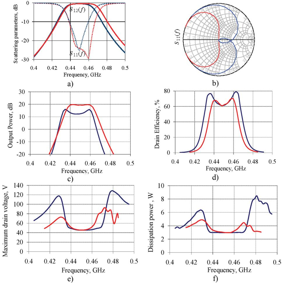
Fig. 6 ADS simulation results of the class-D PA with the ST filter (red curves) and the DT filter (blue curves) as functions of centre frequency: a) - scattering parameters, b) - Smith chart, c) - output power, d) - drain efficiency, e) - maximum drain voltage, f) - dissipated power in the switch
