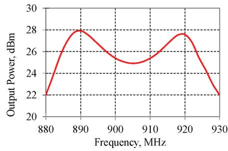
Fig. 7 Typical result for the measured output power of the class-S PA with a DT reconstruction filter, operating for test purposes in class-D over the specified bandwidth around 900 MHz centre frequency
