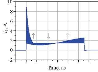
Fig. 4 Numerical simulation results: Variation of the time dependent drain currents (shown by the arrows) for a variation of the ground capacitance from 0 pF to 8 pF (the shape close to rectangular corresponds to  $C_g = 0$ )
