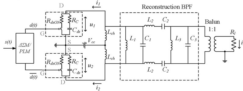
Fig. 1 Building blocks of a class-S power amplifier system comprising a  $\Delta\Sigma$ M or PLM, a push-pull amplifier with an equivalent circuit of the GaN HEMTs ( $C_{ds}$ ,  $R_C$  and  $R_{dsON}$ ) and biasing network (RF chokes  $L_{ch}$  and voltage supply  $V_{cc}$ ), blocking capacitances  $DC_{block}$  and a reconstruction band-pass filter [7]
