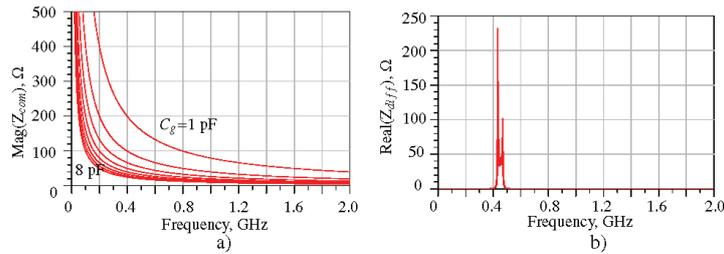
Fig. 3 ADS simulation results of the balanced input BPF at 450 MHz with parasitic capacitances to ground: Magnitude of the input impedance for the common mode (panel a) and input resistance for differential excitation (panel b). The common-mode input magnitude is infinite when  $C_g = 0$  pF
