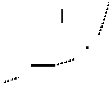
Fig. 3. Skeleton of original image using squares as structuring elements.
