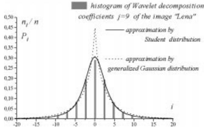
Fig. 1. The approximation of histogram of "Lena" sub-band decomposition based on GGD and StD models.
