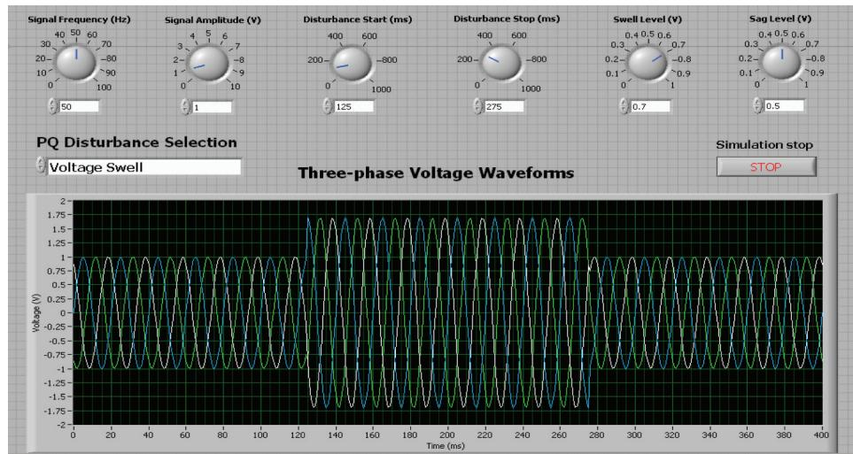
**Fig. 4** LabVIEW presentation of the standard three-phase voltage waveforms with simulation of the voltage swell
