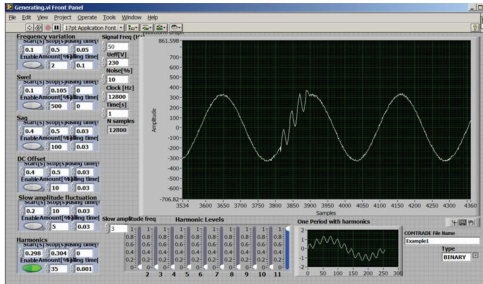
**Fig. 8** Generating of the voltage waveform with short-time transient caused by signal harmonic distortion
