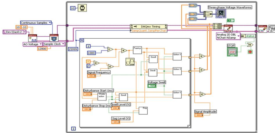
**Fig. 3** One segment of the LabVIEW block diagram corresponding to the virtual instrument for signal generating
