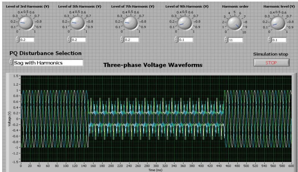
**Fig. 5** Presentation of the standard three-phase voltage waveforms with simulation of the voltage sag and high-order signal harmonics
