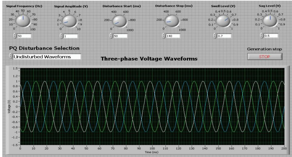
**Fig. 2** Front panel of the LabVIEW virtual instrument for generating and presentation of the standard three-phase voltage waveforms
