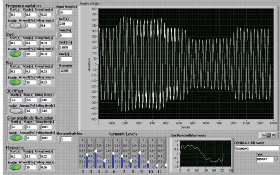
**Fig. 6** Front panel of the signal generator for simulation of the various PQ disturbances in serial combination
