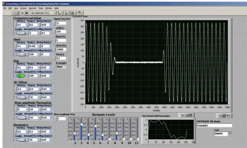
**Fig. 7** LabVIEW front panel of the signal generator for simulation of the waveform with voltage interruption
