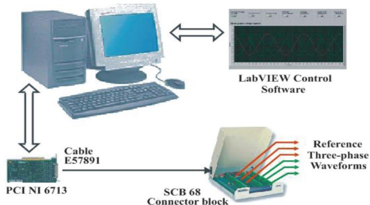
**Fig. 1** Basic hardware configuration of the procedure for signal generating
