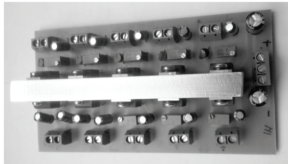
Fig. 5. Realized circuit for DC bias
