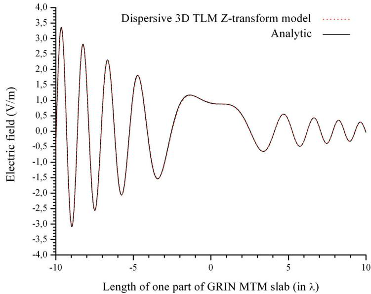
**Fig. 7.** Comparison of the analytical and numerical results for the lossy GRIN MTM slab with hyperbolic tangent profile
