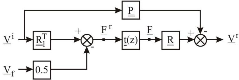
**Fig. 2.** Signal flow diagram of the general algorithm of TLM Z-transform method
