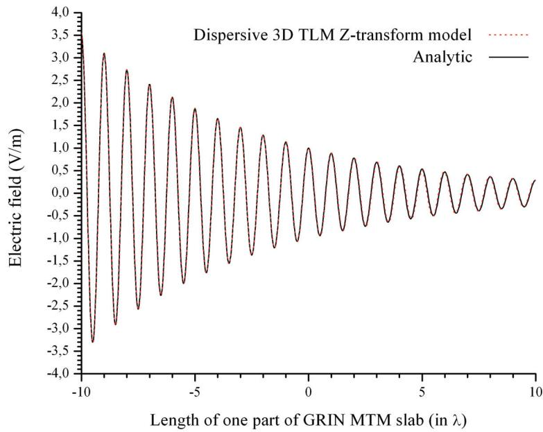
**Fig. 6.** Comparison of the analytical and numerical results for the lossy GRIN MTM slab with abrupt profile
