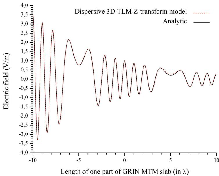
**Fig. 8.** Comparison of the analytical and numerical results for the lossy GRIN MTM slab with cosine profile
