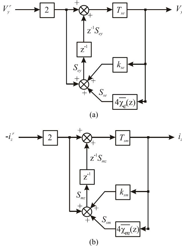
**Fig. 3.** Dispersive 3D TLM Z-transform model for LH MTM: (a) calculation of  $E_y$  in the time-domain, (b) calculation of  $H_z$  in the time-domain
