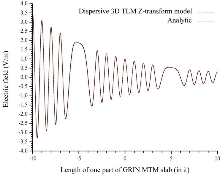
**Fig. 9.** Comparison of the analytical and numerical results for the lossy GRIN MTM slab with linear profile
