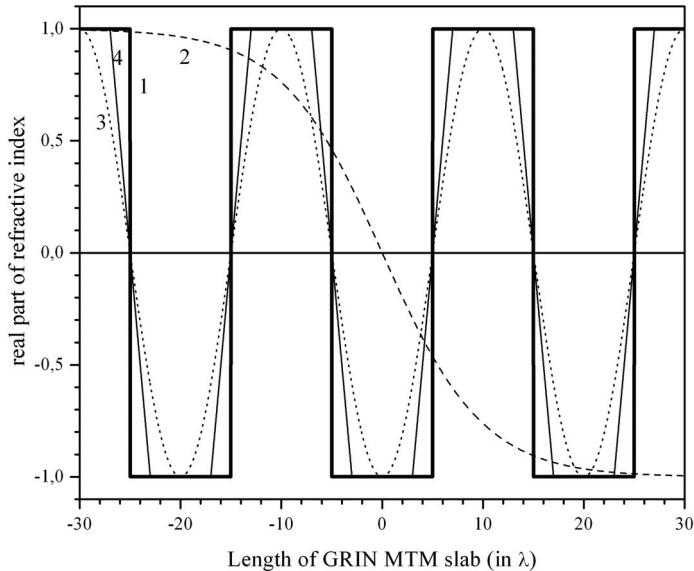
**Fig. 5.** Variation of real part of refractive index across the length of GRIN MTM slab for different profiles: a) abrupt (1), hyperbolic tangent (2), cosine (3) and linear (4)
