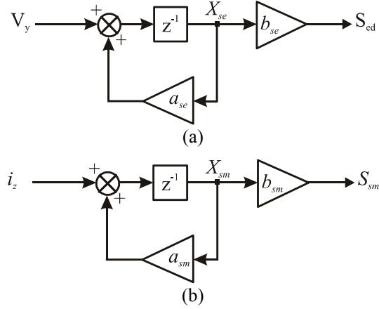
**Fig. 4.** Calculation of: (a) accumulator  $S_{se}$ , (b) accumulator  $S_{sm}$ .
