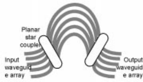
Fig. 6. AWG acting as a 1 \times N demultiplexer or M \times N router.
