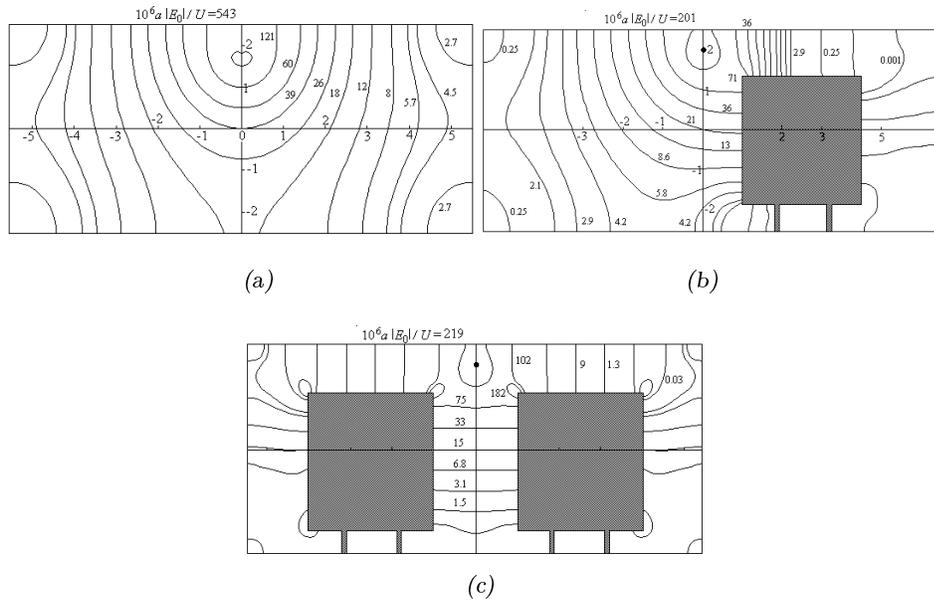
Fig. 14. Equienergetic curves in the vacant bridge (a), in the bridge when a train is in it (b) and in the bridge when two trains are in it (c).
