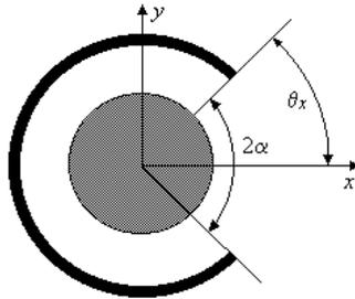
Fig. 16. The slit position of the coaxial line.
