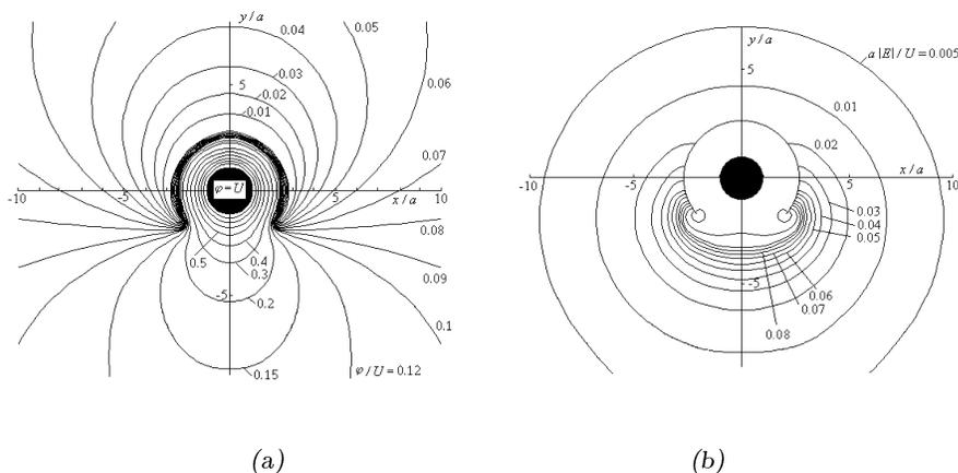
Fig. 3. Equipotential (a) and equienergetic (b) curves of the single coaxial line with axial slit.
