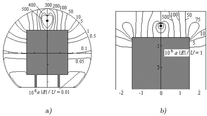
Fig. 8. Equienergetic surfaces of the coax with axial slit in the tunnel a) and in the bridge b), when a train is in it.
