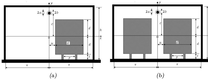
Fig. 10. Mathematical model of bridge when a train is in it (a) and when two trains (b) are in it.
