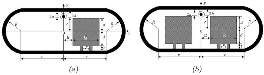
Fig. 9. Mathematical model of tunnel when a train is in it (a) and when two trains (b) are in it.
