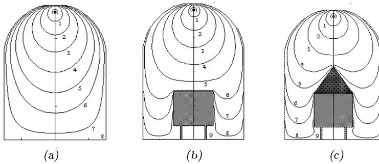
Fig. 17. Equipotential curves (Table 7) in vacant mine pit (a), when empty wagon is inside (b) and when loaded wagon is inside (c).
