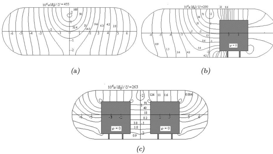
Fig. 13. Equienergetic curves in the vacant tunnel (a), in the tunnel when a train is in it (b) and in the tunnel when two trains are in it (c).
