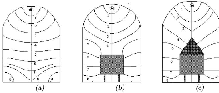
Fig. 19. Equienergetic curves (Table 9) in vacant mine pit (a), when empty wagon is inside (b) and when loaded wagon is inside (c).
