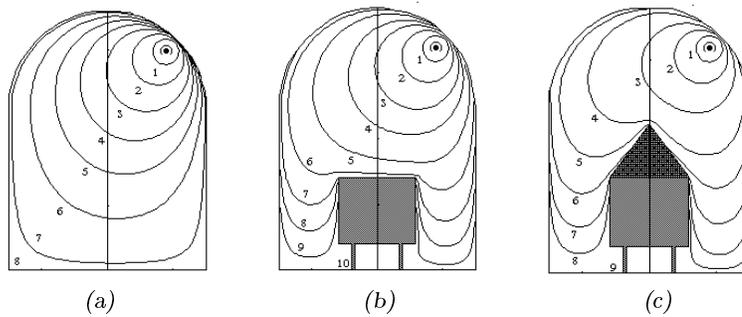
Fig. 18. Equipotential curves (Table 8) in vacant mine pit (a), when empty wagon is inside (b) and when loaded wagon is inside (c).
