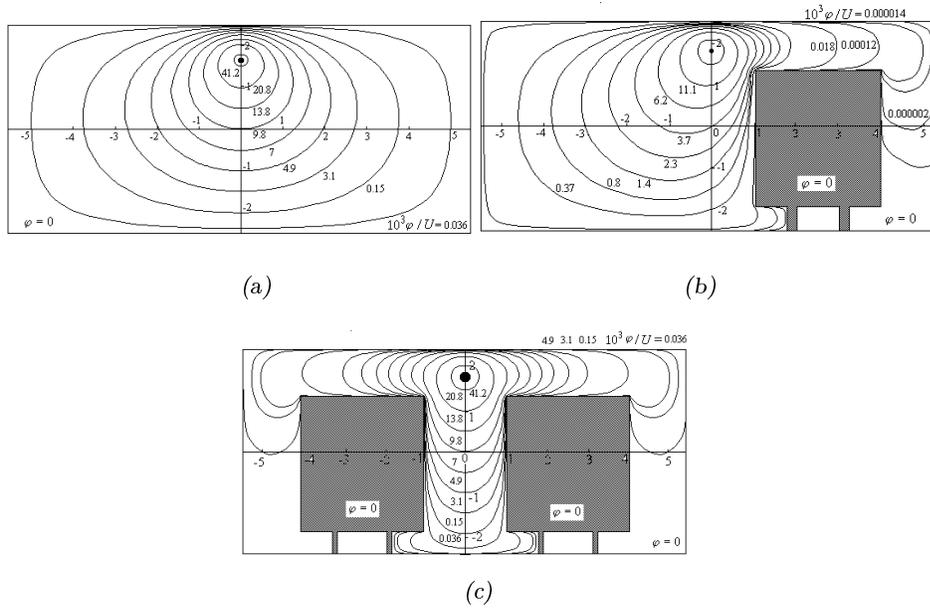
Fig. 12. Equipotential curves in the vacant bridge (a), in the bridge when a train is in it (b) and in the bridge when two trains are in it (c).
