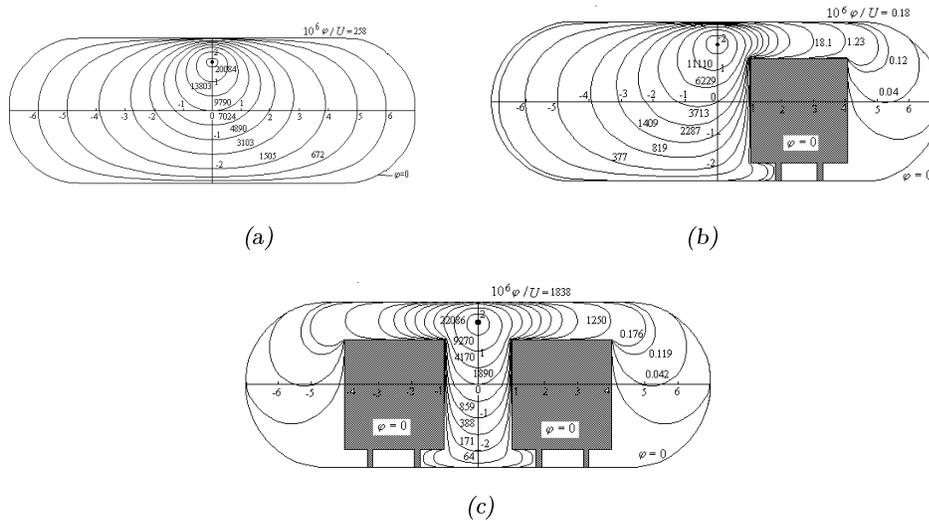
Fig. 11. Equipotential curves in the vacant tunnel (a), in the tunnel when a train is in it (b) and in the tunnel when two trains are in it (c).
