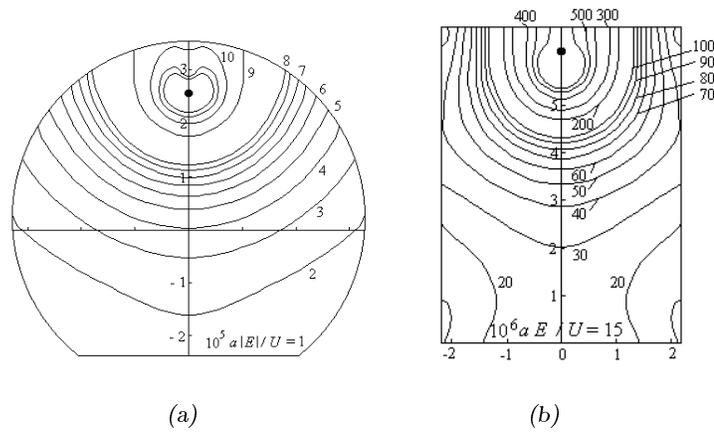
Fig. 6. Equipotential surfaces of the coax with axial slit in the vacant tunnel (a) and in the vacant bridge (b).
