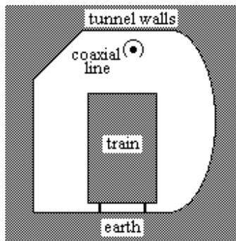
Fig. 1. Cross section of conducting cavity representing mathematical model.
