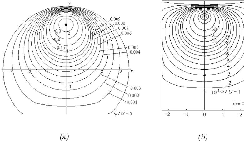
Fig. 5. Equipotential curves of the coax with axial slit in the vacant tunnel (a) and in the vacant bridge (b).
