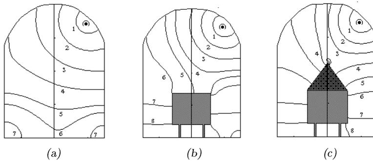
Fig. 20. Equienergetic curves (Table 10) in vacant mine pit (a), when empty wagon is inside (b) and when loaded wagon is inside (c).
