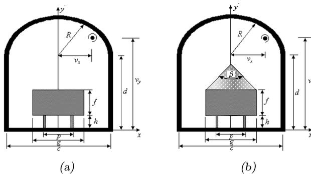
Fig. 15. Mathematical model of mine pit when empty wagon (a) and when loaded wagon (b) is inside.
