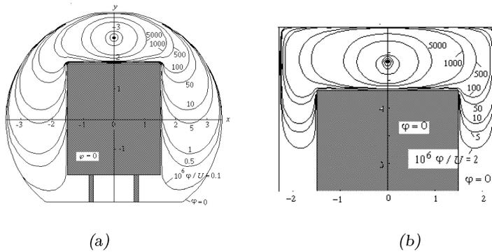
Fig. 7. Equipotential curves of the coax with axial slit in the tunnel (a) and in the bridge (b), when a train is in it.
