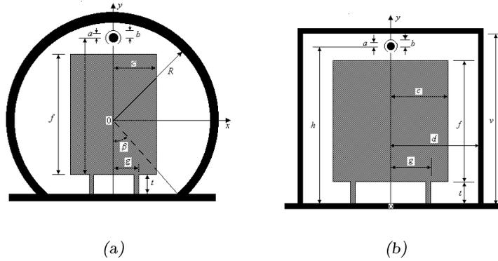
Fig. 4. One track tunnel (a) and one track bridge (b), when a train is in it.
