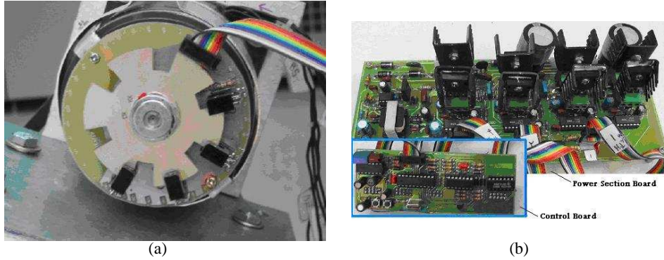
Fig. 6. ((a) Sensors board mounted on the 8/6 SRM shaft, and (b) 8/6 SRM drive for measurement purpose.
