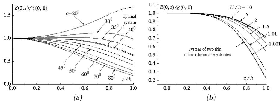
Fig. 6. The ratio  $E(0, z)/E(0, 0)$  on the system axis,  $r = 0$ .
