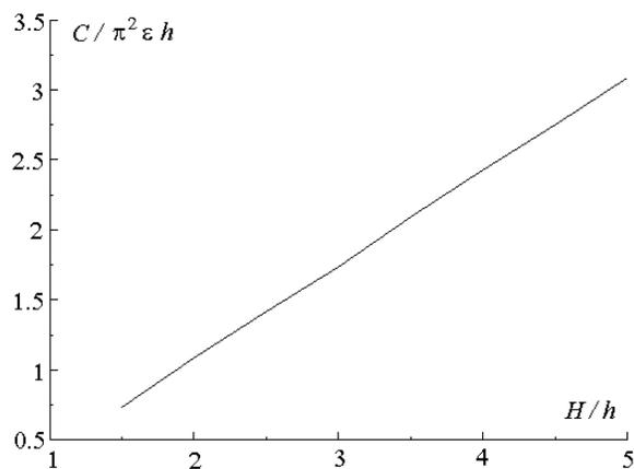
Fig. 10. Capacitance of optimal system for different ratio  $H/h$ .
