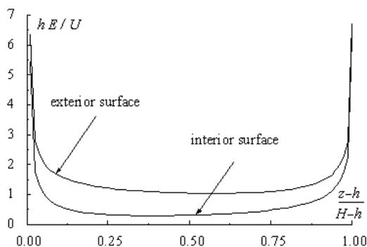
Fig. 9. Electric field strength on the electrode surface for optimal system for  $\delta = 0$ .
