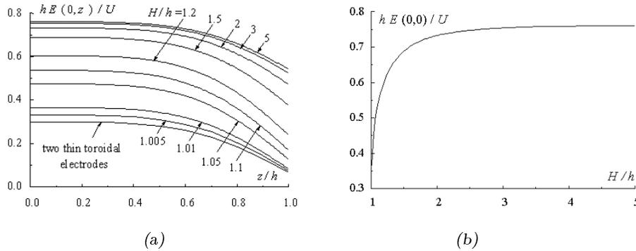
Fig. 7. Electric field strength for the primary cell of the first kind.
