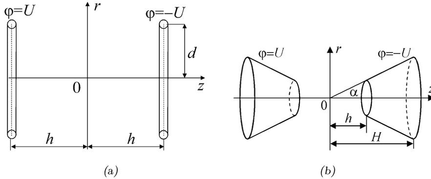
Fig. 1. The primary cell for generating homogeneous electric field.
