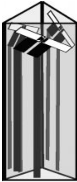
Fig. 2. The screen printed probe. The LID encapsulated detector diode is mounted into the gap of the silver printed dipole. The carbon printed resistive lines are connected to the wings of the dipole via chip resistors.
