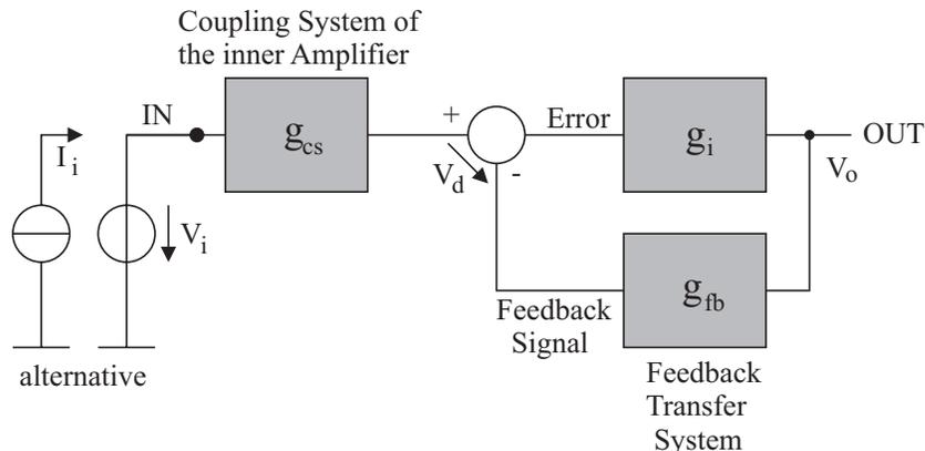
Fig. 1. Schematic circuit diagram of a closed-loop amplifier
