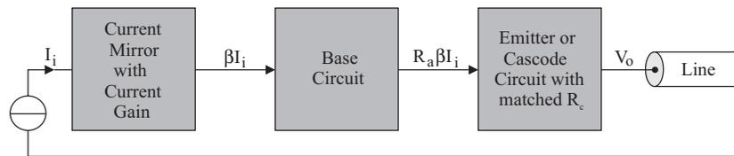
Fig. 4. Proposed transceiver circuit without TISs and Efs [6]
