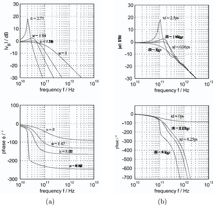
Fig. 2. Frequency response in the case of destabilisation by (a) multiple poles  $n$ , (b) delay times  $t_d$
