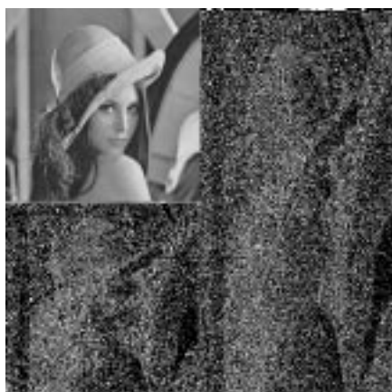
Figure 6. Nonseparable DWT decomposition of "Lena" image "packed" for compact use of memory.
