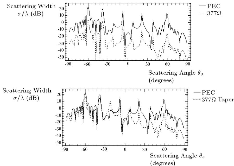
Figure 4. Bistatic scattering width ten strip array on grounded dielectric slab (freq=12GHz,  $W = 5.08\text{cm}$ ,  $D = W$ ,  $d = 0.07874\text{cm}$ ,  $\epsilon_r = 2.33$ , loss tangent=0.001,  $\theta = -60.0^\circ$ ,  $\theta_s = 60.0^\circ$ ).
