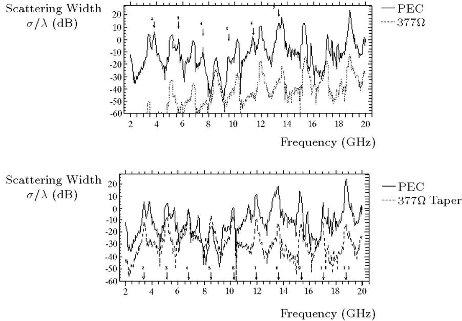
Figure 3. Comparison of calculated monostatic scattering width as a function of frequency for ten strip array on grounded dielectric slab ( $W = 5.08\text{cm}$ ,  $D = W$ ,  $d = 0.07874\text{cm}$ ,  $\epsilon_r = 2.33$ ,  $\text{loss tangent} = 0.001$ ,  $\theta_i = -60.0^\circ$ ,  $\theta_s = 60.0^\circ$ ).
