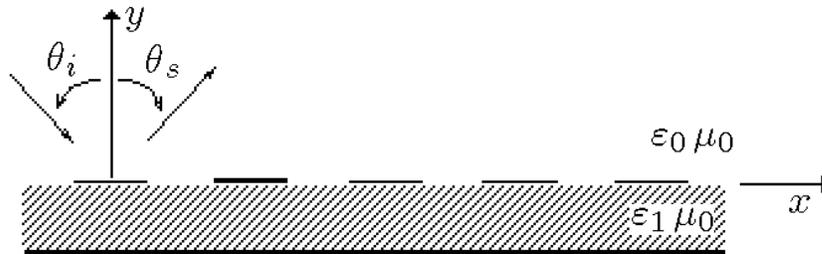
Figure 1. The geometry of the finite strip array supported by a dielectric slab.
