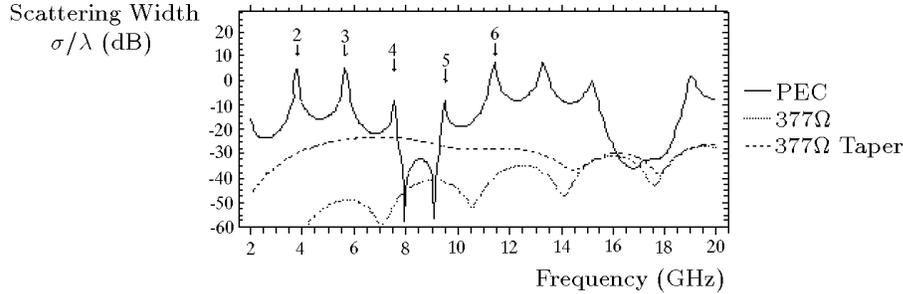
Figure 2. Comparison of calculated monostatic scattering width as a function of frequency for single strip on grounded dielectric slab ( $W = 5.08\text{cm}$ ,  $d = 0.07874\text{cm}$ ,  $\epsilon_r = 2.33$ , loss tangent=0.001,  $\theta_i = -60.0^\circ$ ,  $\theta_s = 60.0^\circ$ ).
