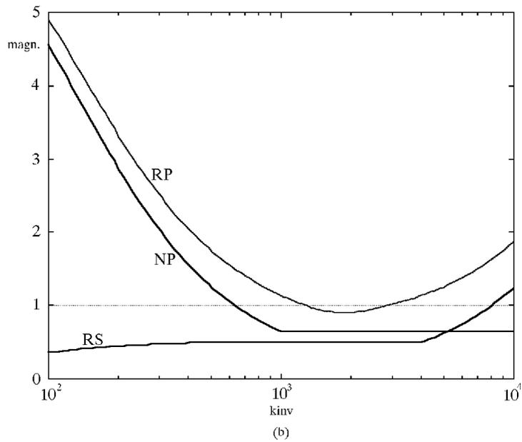
Figure 5. Inversion-based controller design for a) unstructured and b) structured model uncertainty.  $RP$ ,  $RS$  and  $NP$  measure are shown as a function of the adjustable parameter  $k_{inv}$ ,  $RP(k_{inv})$ ,  $RS(k_{inv})$ ,  $NP(k_{inv})$ .
