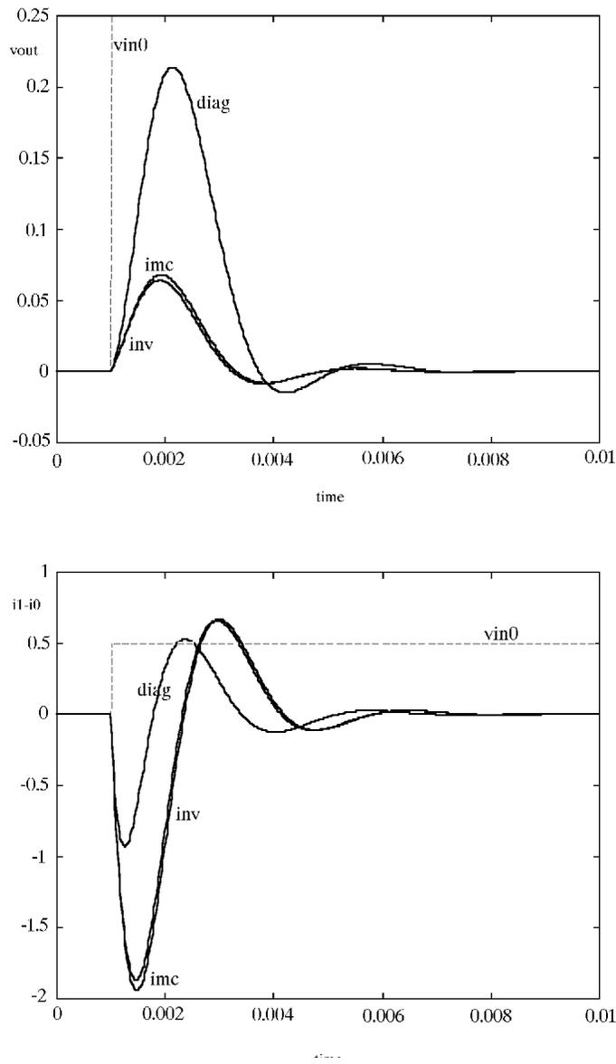
Figure 15(b). The response to a step-source ( $e_1$ ) disturbance acting on unit 1.
