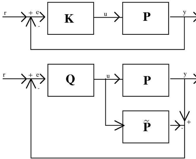
Figure 11. a) The standard and b) the IMC feedback structure.
