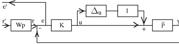
Figure 3. The block diagram of the feedback system with setpoint changes as external inputs.
