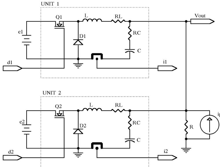
Figure 1. Two parallel operating (buck) switch-mode power supplies.
