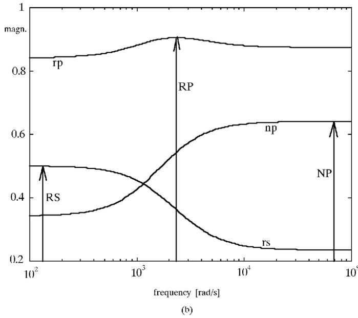
Figure 6. Inversion-based controller. The frequency responses of  $rp(\omega)$ ,  $rs(\omega)$ ,  $np(\omega)$  a) unstructured and b) structured model uncertainty.
