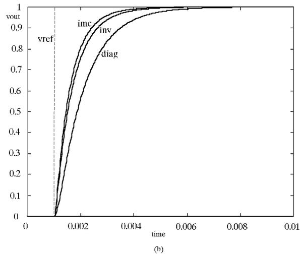
Figure 14. The response to the output voltage setpoint change,  $\tilde{P} \neq P$ .
