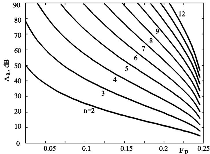
Fig. 3. Design curves for half-band elliptic IIR filters.
