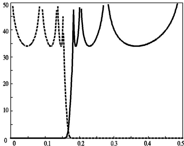
Fig. 7. Attenuations of the 7th-order complementary filters:  $F_{3\text{ dB}} = 0.5/3$ ,  $F_a = 0.18$ ,  $n=7$ .
