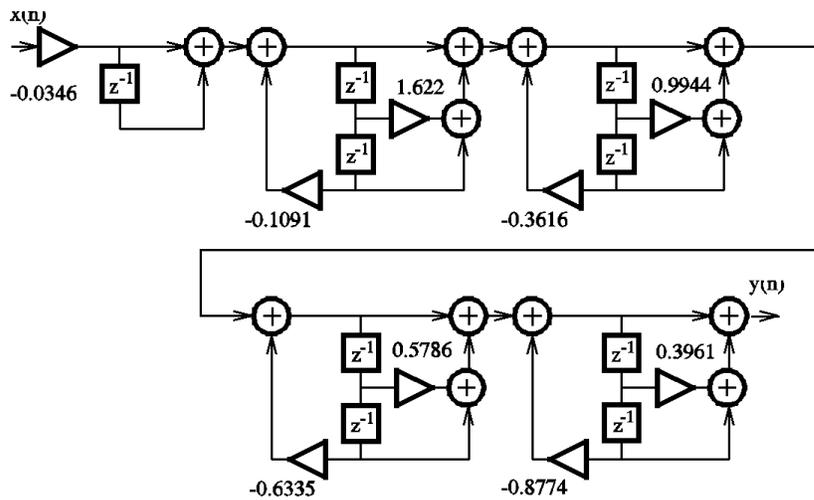
Fig. 5a. Cascaded realization of 9th-order half-band filter.
