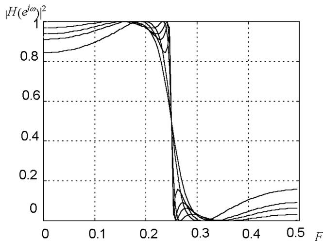
Fig. 2. A family of amplitude characteristics of the fourth-order half-band filters
