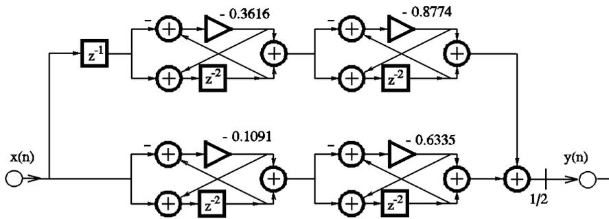
Fig. 5c. Realization of half-band filter based on a parallel connection of two allpass networks
