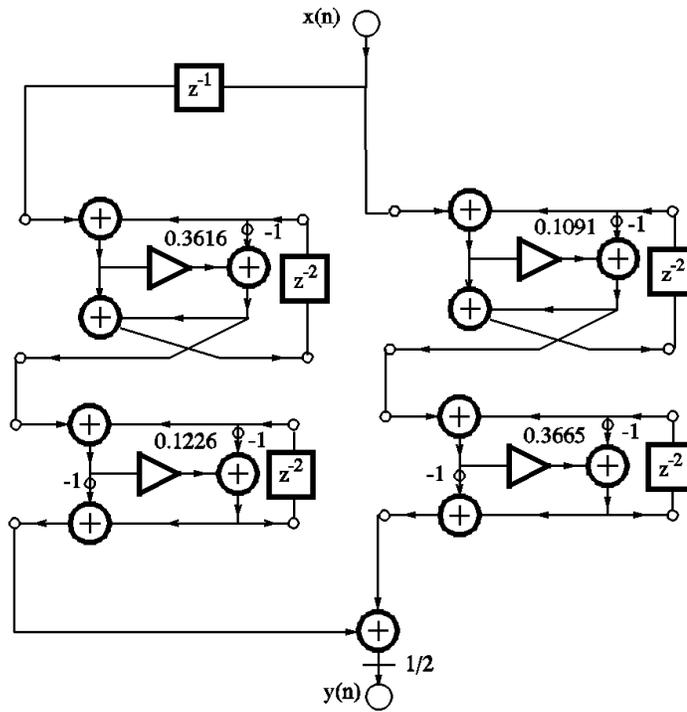
Fig. 5d. Wave digital filter realization.
