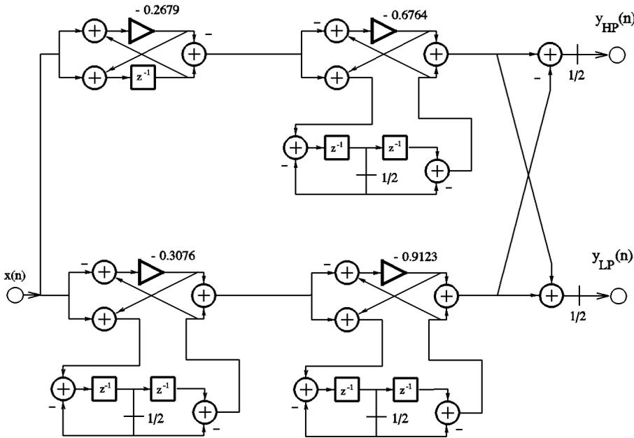
Fig. 6. Realization of the 7th-order complementary low-pass,  $y_{LP}$ , and high-pass filter  $y_{HP}$ .
