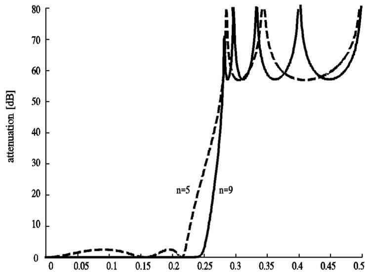
Fig. 4. Attenuation characteristics of the 9th-order half-band filter and of the standard elliptic 5th-order filter.
