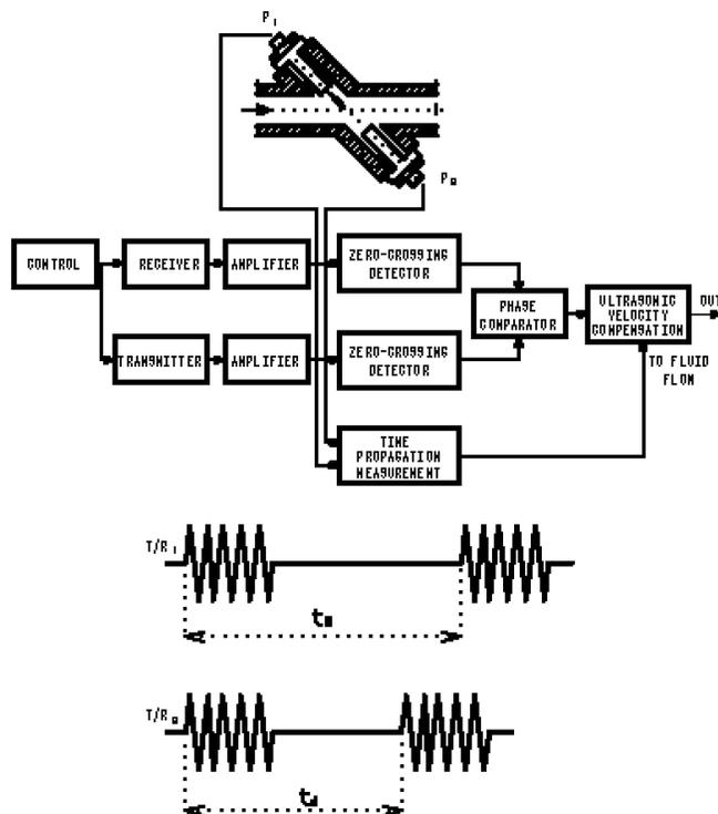
Fig. 6. Burst phase-difference method
