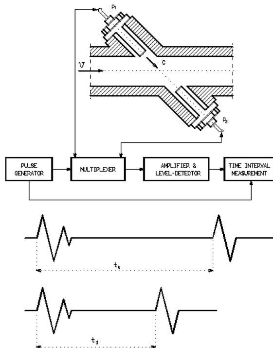
Fig. 4. Sequential direct time measurement
