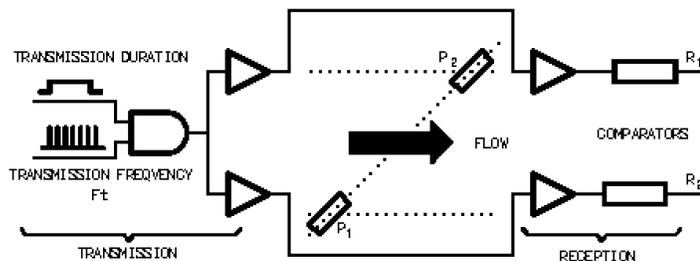
Fig. 5. Simultaneous fluid flow measurement
