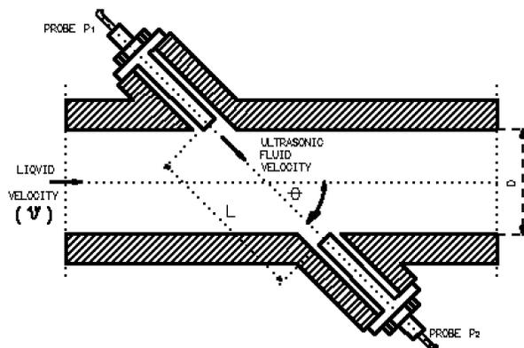
Fig. 1. Physical position of the flowmeter's ultrasonic probes
