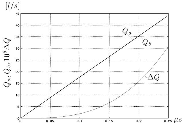
Fig. 2. Flow volume quantity  $Q$  and error approximation  $\Delta Q$  in the function of time-propagation  $\Delta t$
