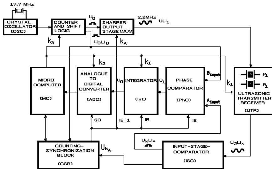
Fig. 8. Global block scheme of the flowmeter
