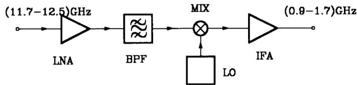
Fig. 1. Block diagram of a typical DBS down converter.
