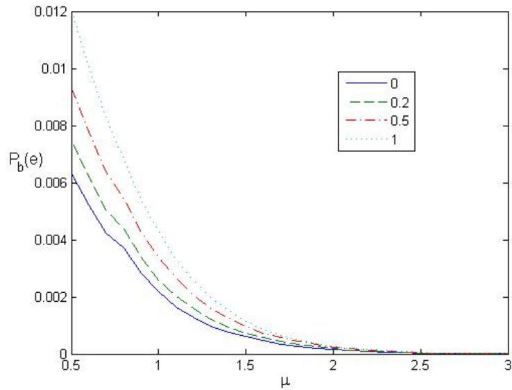
**Fig. 3** Bit error rate for SSC/MRC combiner versus parameter  $\mu$  for  $\sigma = 1$ , for different values of  $\rho$
