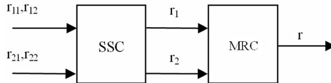
**Fig. 1** Model of the SSC/SC combiner with two inputs at two time instants
