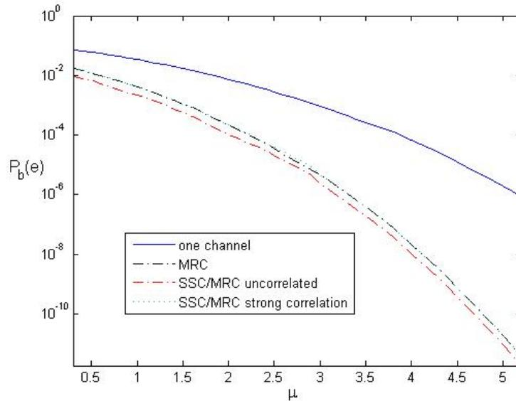
**Fig. 2** Bit error rate for different types of combiners versus parameter  $\mu$  for  $\sigma = 1$
