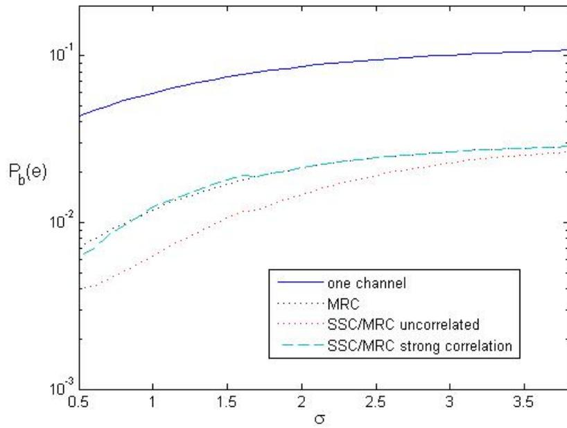
**Fig. 4** Bit error rate for different types of combiners versus parameter  $\sigma$  for  $\mu = 0.5$
