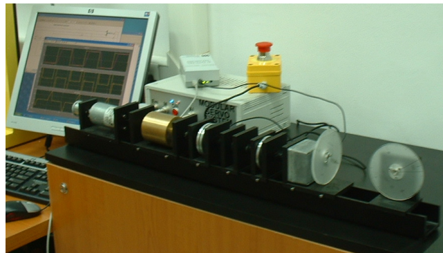
Fig. 11. INTECO modular servo laboratory setup
