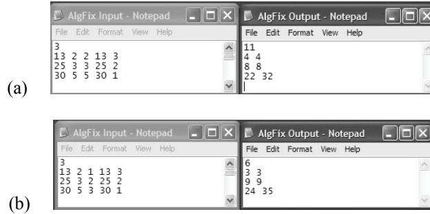
Fig. 4 Input and output file of realized software for (a) case I - system recovers executing task again (b) case II - system recovers executing alternative task
