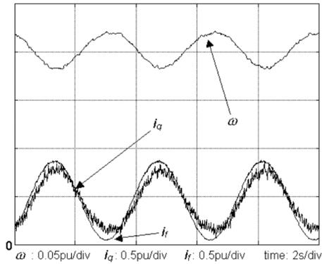
Fig. 7 Speed transient and torque command for sinusoidal load torque disturbance when the local loop of the DOB structure is disconnected.
