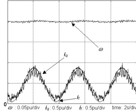
Fig. 8 Speed transient and torque command for sinusoidal load torque disturbance when the local loop of the DOB structure is connected.
