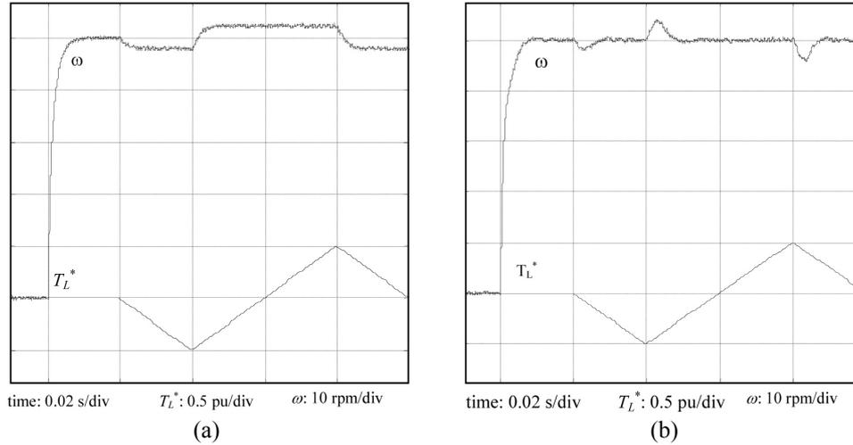
Fig. 2. Rejection of a ramp profiled disturbance: (a) with the standard DOB, (b) with the proposed DOB modified for ramp disturbances.
