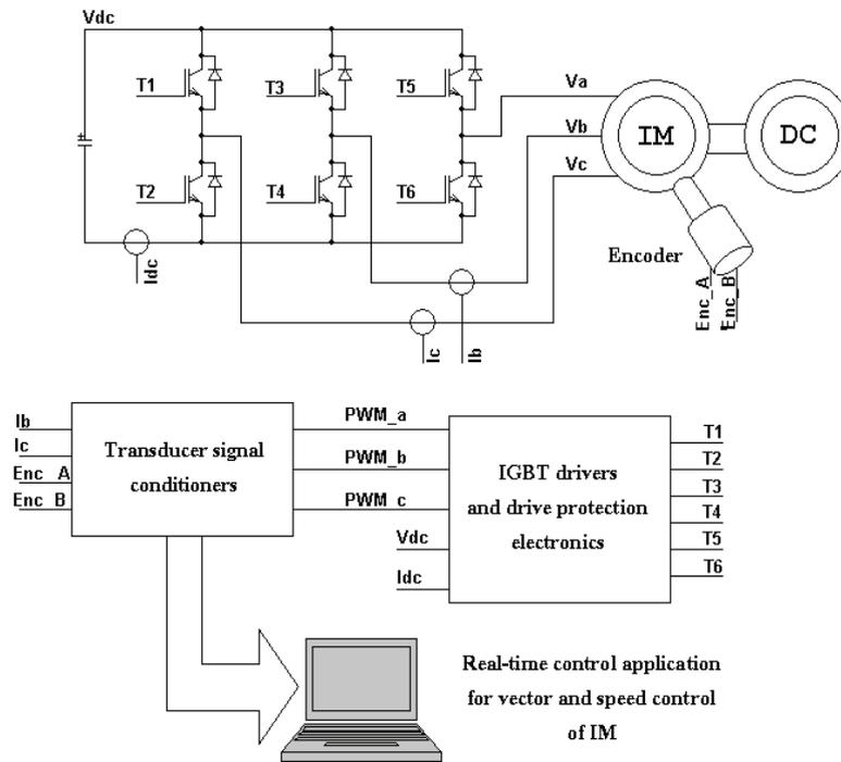
Fig. 4. Experimental setup.
