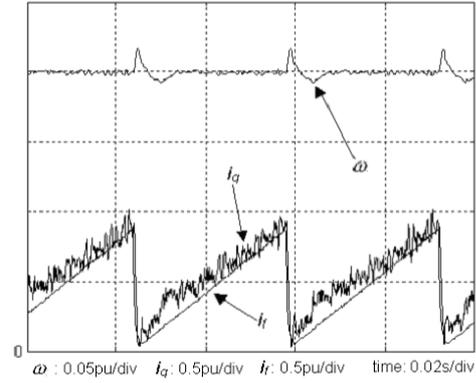
Fig. 6. Speed transient and torque command for combined ramp load torque disturbance with included DOB control section.
