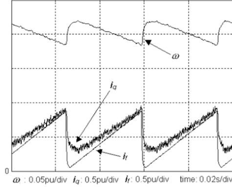
Fig. 5. Speed transient and torque command for load torque disturbance with excluded DOB control section.
