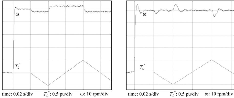
Fig. 3. Rejection of a ramp profiled disturbance in the case when  $\hat{C}_m = 3C_m$  :
