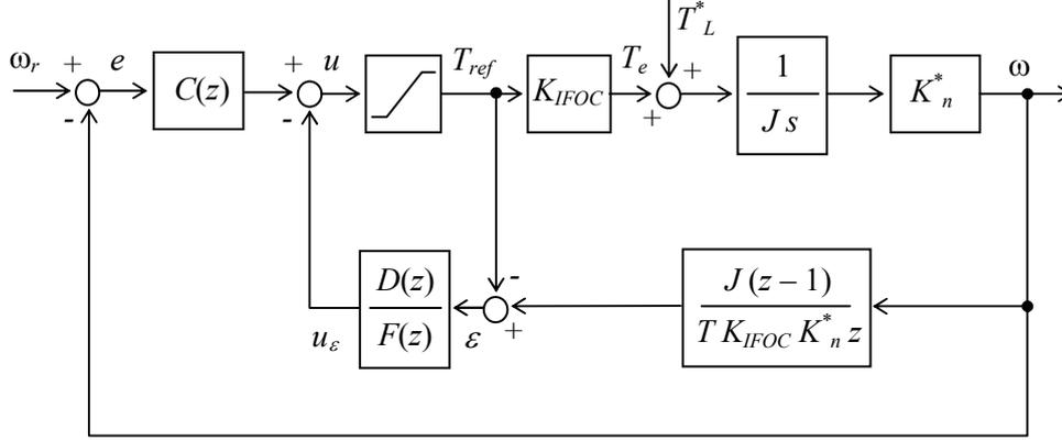
Fig. 1 DOB based speed-controlled drive.
