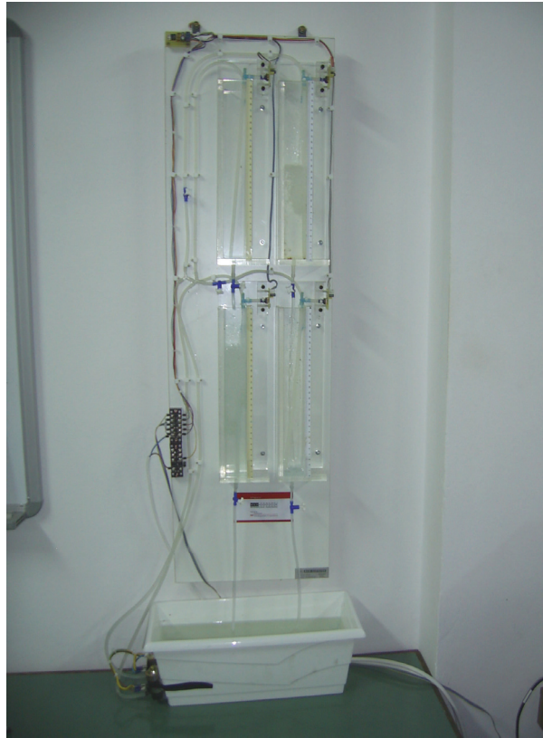
Fig 3 Coupled water tanks experimental setup
