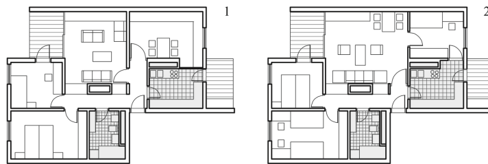
Fig. 12. Housing unit with technical blocks positioned along the wall between two apartments and common building area, [13]
