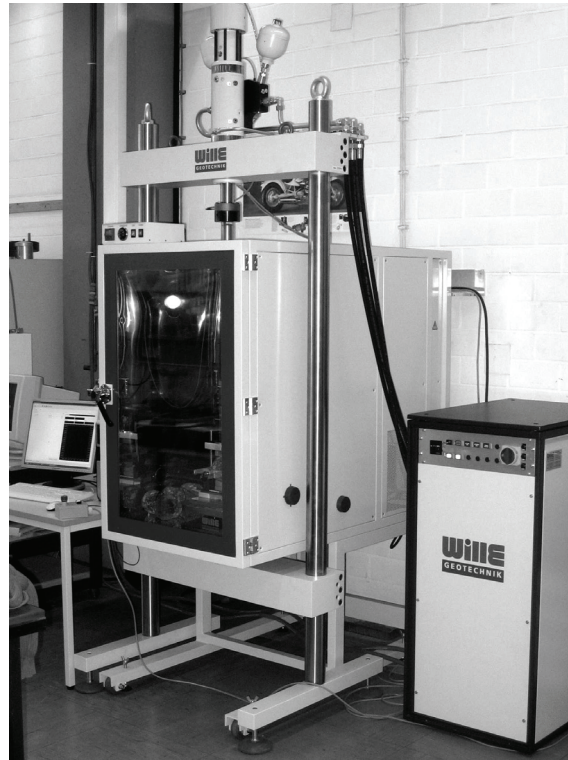
Fig. 5. Servo-hydraulic dynamical testing device for determination of stiffness, cyclic compression test, and fatigue resistance according to EN 13108-26:2004 [12], EN 13108-25:2005 [13], and EN 13108-24:2004+A1:2007 [15].
