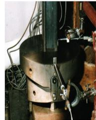
Fig. 2. Spherical bearing - Amsler type
