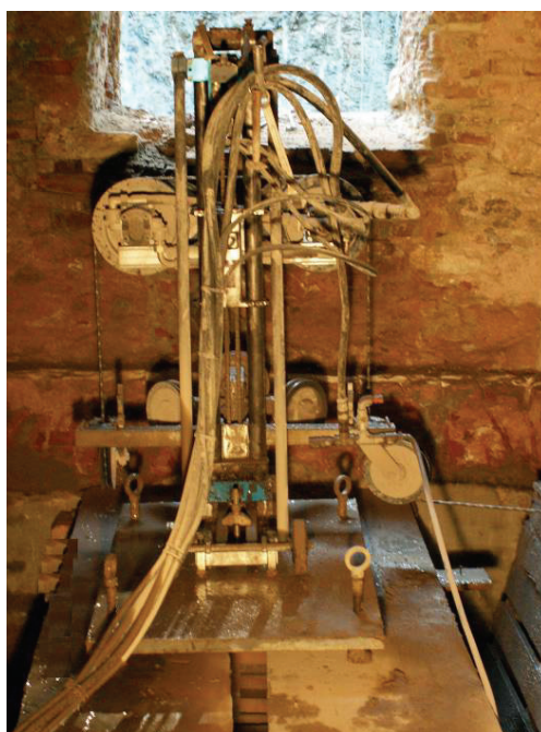
Fig. 11. Part of regulation turbo machine used for circular motion of the beaded cutting wire
