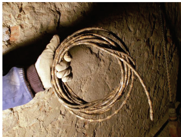
Fig. 2. Special beaded wire for masonry cutting.
