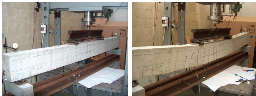
Fig. 8 Experimental setup – prior to loading and under loading.
