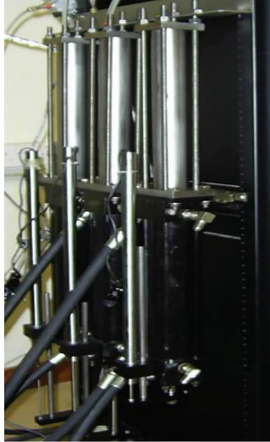
Fig. 3 Pressure system for hollow cylinder apparatus
