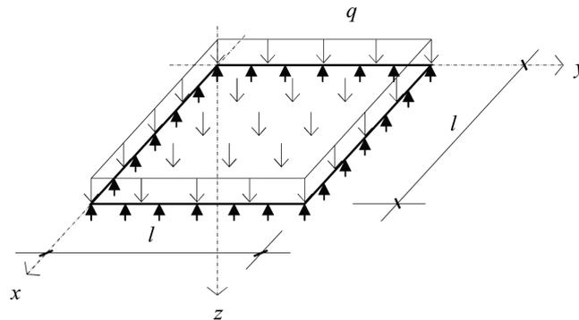
Fig. 6 Calculation model of simply supported square plate
