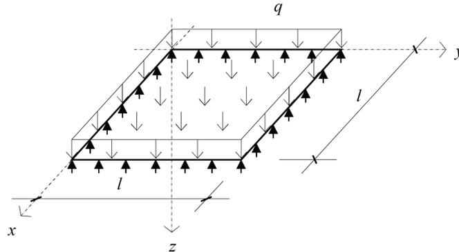
Fig. 8 Calculation model of simply supported square plate
