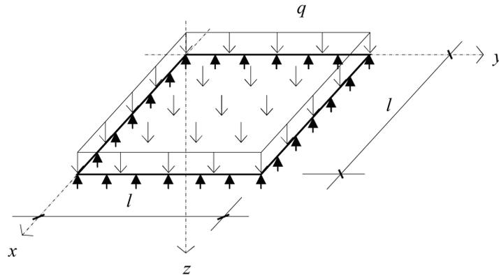
Fig. 2 Calculation model of simply supported square plate
