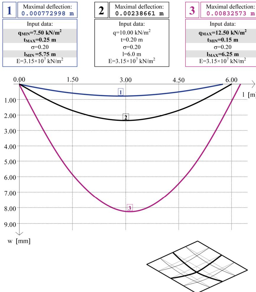
Fig. 9 Diagram of maximal plate deflections (Numerical example 4)
