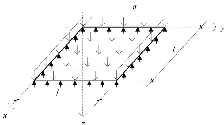
Fig. 10 Calculation model of simply supported square plate
