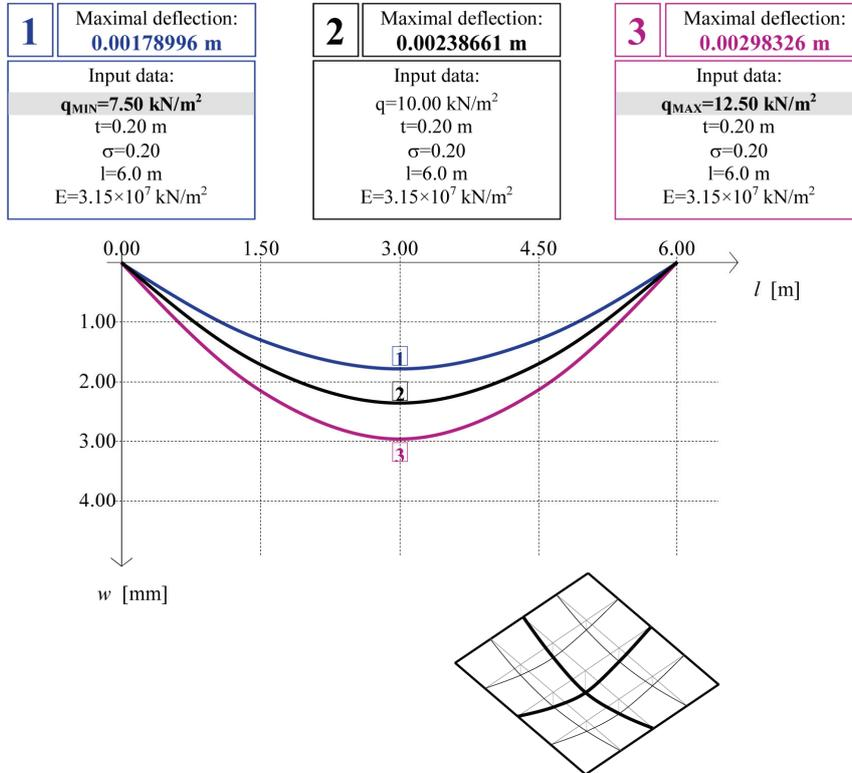
Fig. 5 Diagram of maximal plate deflections (Numerical example 2)
