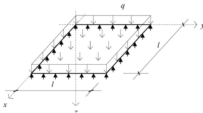
Fig. 4 Calculation model of simply supported square plate
