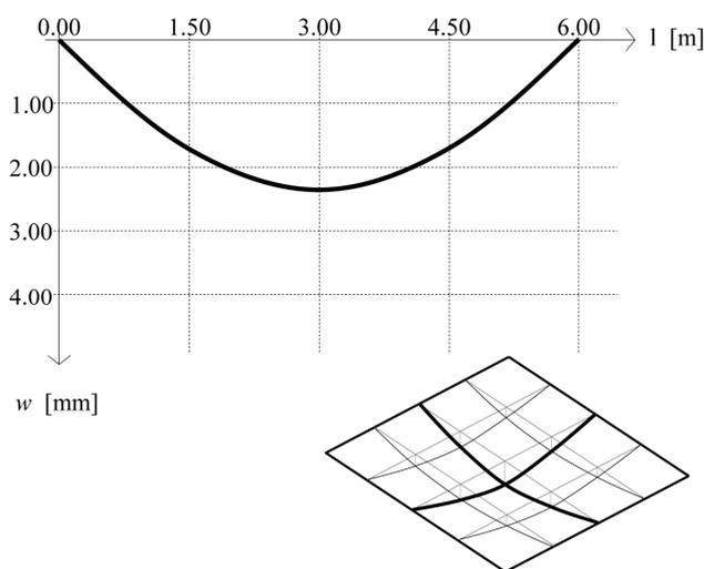
Fig. 3 Diagram of maximal plate deflections (Numerical example 1)
