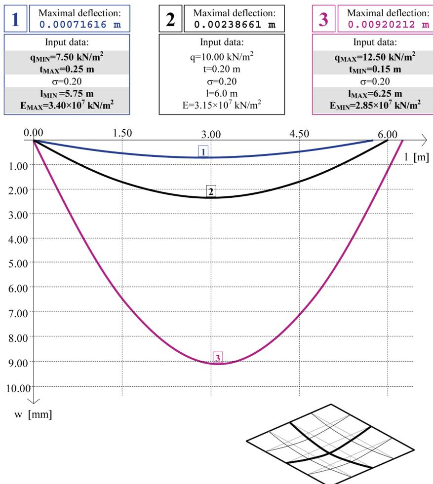
Fig. 11 Diagram of maximal plate deflections (Numerical example 5)
