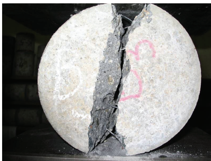
Fig. 5 Steel fibers continue to bridge the crack after the breakage of the specimen
