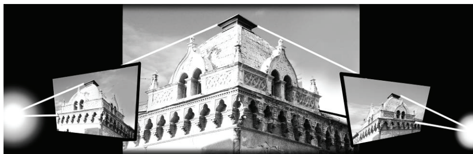
Fig. 1. Minimum two photographs are basis for terrestrial photogrammetry
