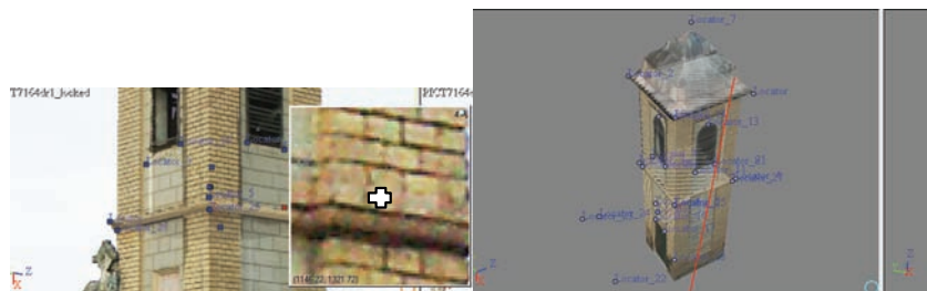
Fig. 4. Epipolar trace on model of bell tower in Apatin in Donje groblje.
