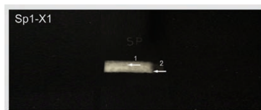
Fig. 6. X-ray image of the pieces of the wall tie brace originating from the Sándor palace at Budapest. The horizontal lines indicating the locations of the longitudinal welds are visible at several locations in the sample; at the half (arrow 1) and at the lower fifth (arrow 2.).
