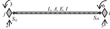
Fig. 1. Model of member with rotational semi-rigid connections on the ends ( S_{rj} , S_{rk} – rotational stiffness)
