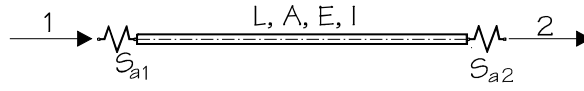
Fig. 2. Model of member with axial flexibility on the ends ( S_{aj} , S_{ak} – axial stiffness)
