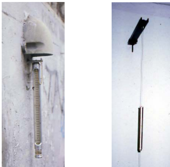
Fig. 1. Short rods fixed on the wall and connected with a steel wire
