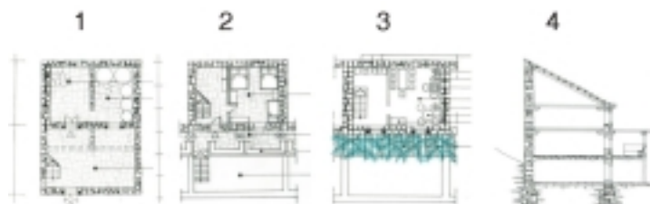
Fig. 4. Basis of the typical house of Pastrovici: 1. Basis of the upper floor, 2. Basis of the ground floor, 3. Basis of the cellar, 4. Cross-section
